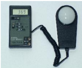
Fig. A2:45. Standard Light Meter showing a reading of inside daylight at 850 Lux.
