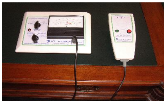
Fig. 1. Infrared Desktop Diagnostic Scanner: Meter console (left) and hand-held scanner (right). The meter console is equipped with 'sensitivity' and 'function' control knobs.
