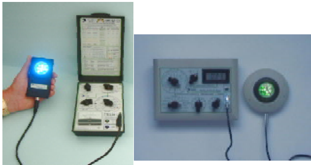
Fig. A2:46 & 47. A Matrix of 12 super bright white Light Emitting Diodes. The Output was only 76 Lux at 10 Centimetre when filled with Emerald and Sapphires with a Green Filter.
