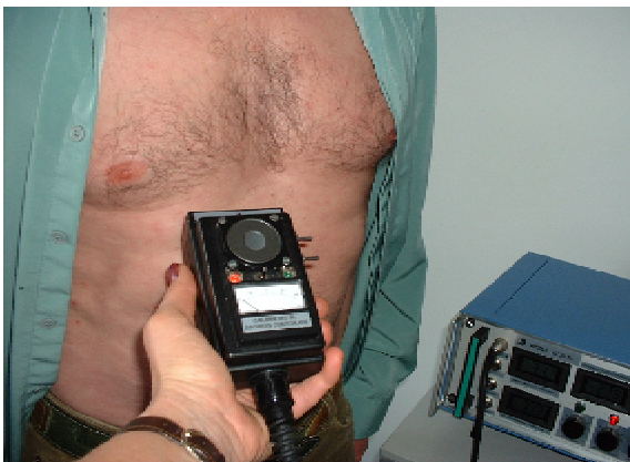
Fig. A2:4. Scanning infrared emissions using an early prototype infrared scanner calibrated against platinum temperature references.
